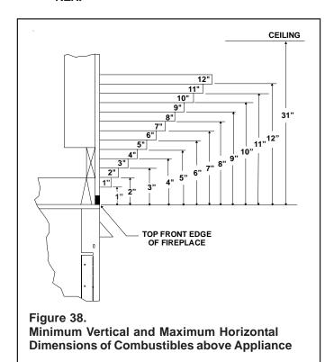
CAUTION: IF JOINTS BETWEEN THE FINISHED WALLS AND THE APPLIANCE SURROUND (TOP AND SIDES) ARE SEALED, A 300° F. MINIMUM SEALANT MATERIAL MUST BE USED. THESE JOINTS ARE NOT REQUIRED TO BE SEALED. ONLY NON-COMBUSTIBLE MATERIAL (USING 300° F. MINIMUM ADHESIVE, IF NEEDED) CAN BE APPLIED AS FACING TO THE APPLIANCE SURROUND. SEE THE DIAGRAM BELOW.
